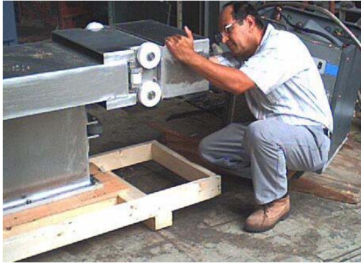
Unpacking the collector (the moving part of the linear joint).
