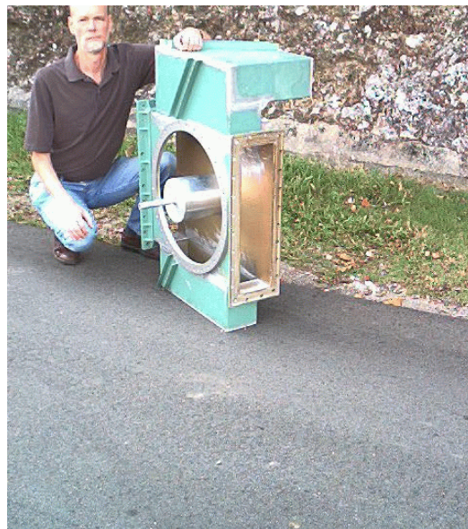
Dome turnstile junction. Side ports are half-height waveguide. Side shorts are fixed. Note concentric post tuning structure.
