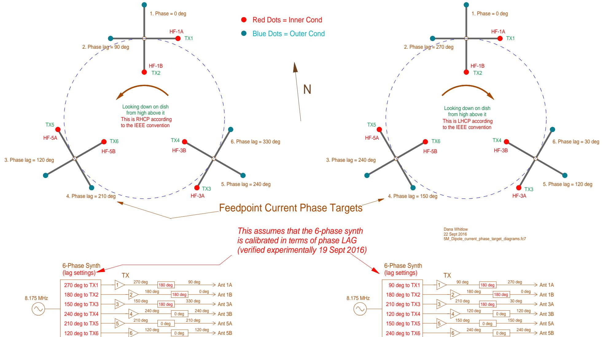
5-MHz HF DIPOLE CURRENT PHASE TARGETS FOR CIRC POLARIZATION
