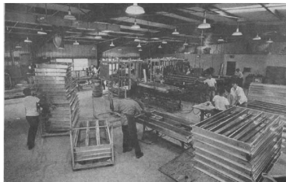
The rugged terrain of the area makes overland trucking of large objects difficult, so the aluminum panels are assembled in a factory right at the telescope site.
