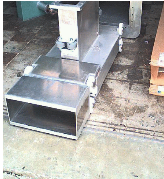
Collector (upside down) Main body and output stack are half-height waveguide. Input scoop is a \lambda/4 matching transformer. Choke joint cavities at top and bottom of scoop prevent blow-by.
