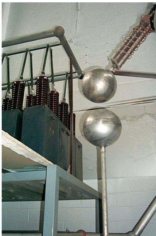
Crowbar discharge balls. Capacitors at left are part of the capacitor bank.
