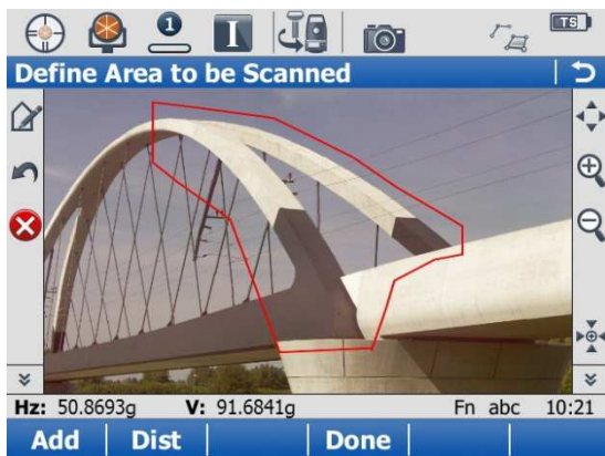
Figure 18 Polygonal scan area definition using the onboard live video stream
