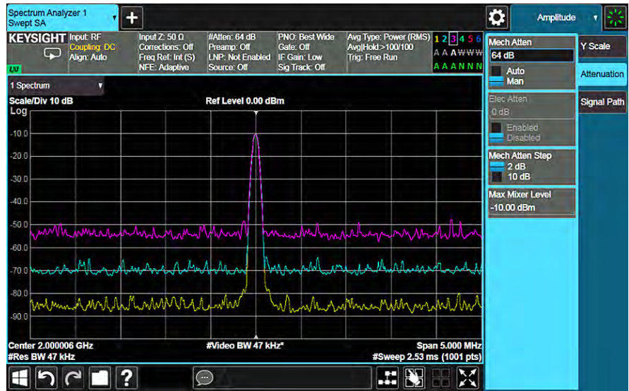
Figure 5-1. In modern signal analyzers, reference levels remain constant when you change input attenuation
