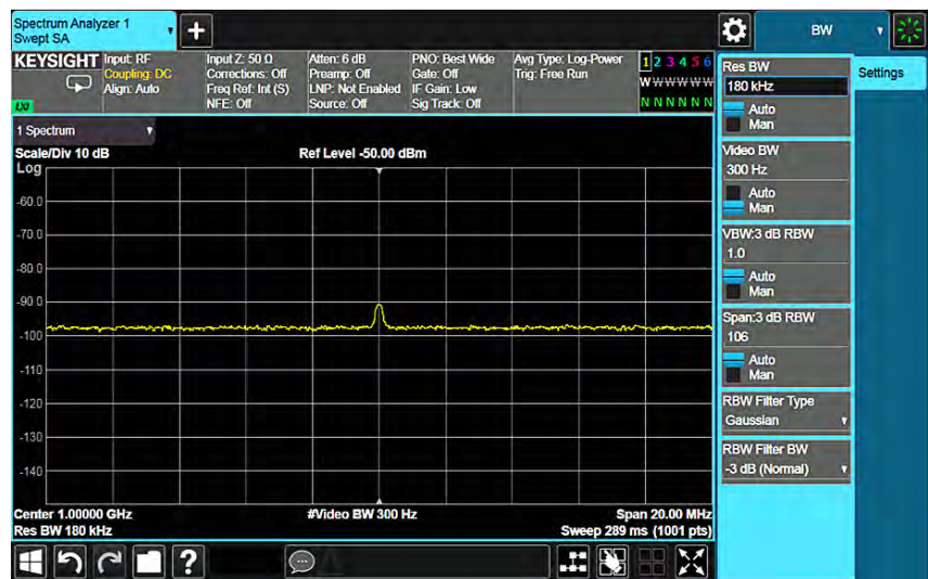
Figure 5-3. Video filtering makes low-level signals more discernible
