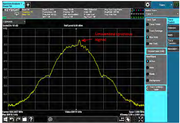
Figure 2-37. Frequency domain view of the GSM signal with 2 time slots “on” showing an unwanted spurious signal present in the spectrum.
