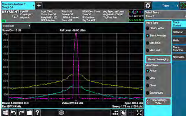
Figure 2-12a. Phase noise performance can be optimized for different measurement conditions
