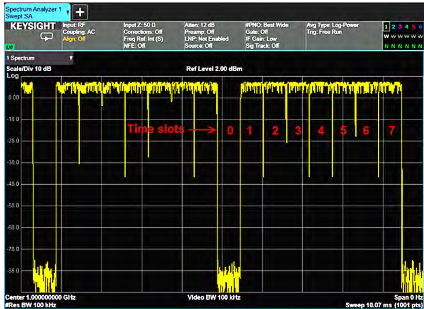
Figure 2-35. A TDMA format signal (in this case, GSM) with 8 time slots, time slot zero is "off".
