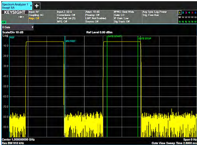
Figure 2-38. Time gating is used to look at the spectrum of the GSM time slot 3.
