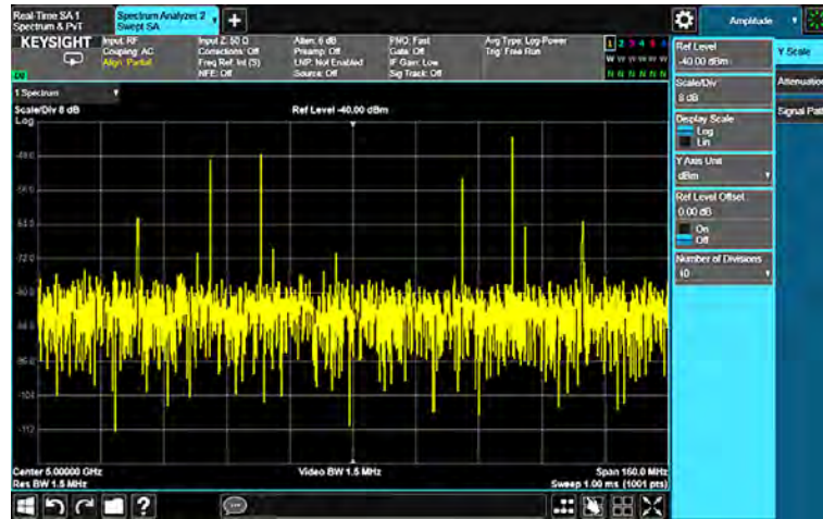
Figure 8-7. Even when you use fast sweeps and max hold over a period of many seconds, the swept spectrum analyzer view of the radar signal is not very informative
