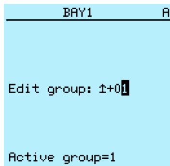
Figure 17: Last digit is active and it can only be increased
