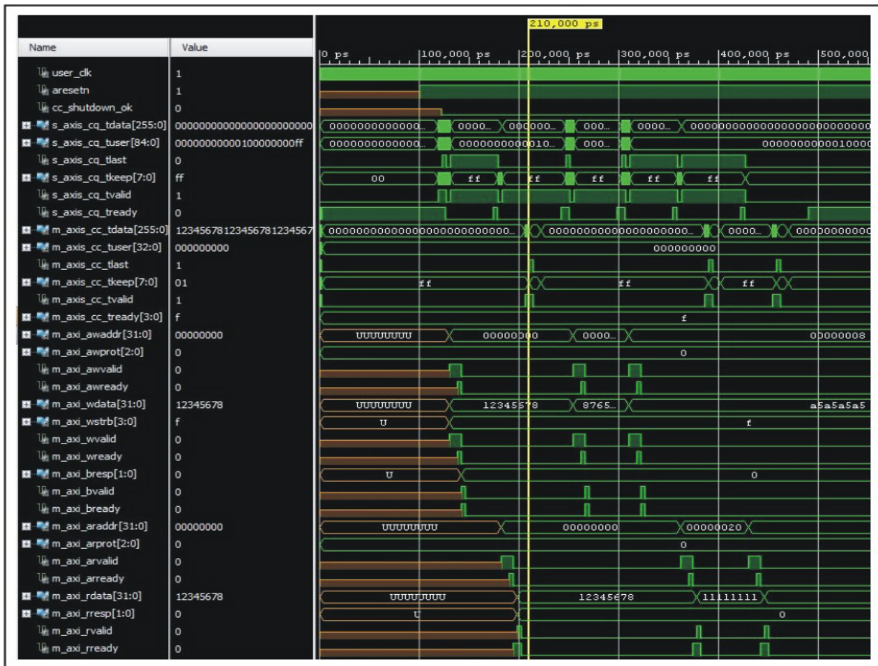
Figure 5-3: PCI Express to AXI4-Lite Bridge Core Test Bench Simulation Output
