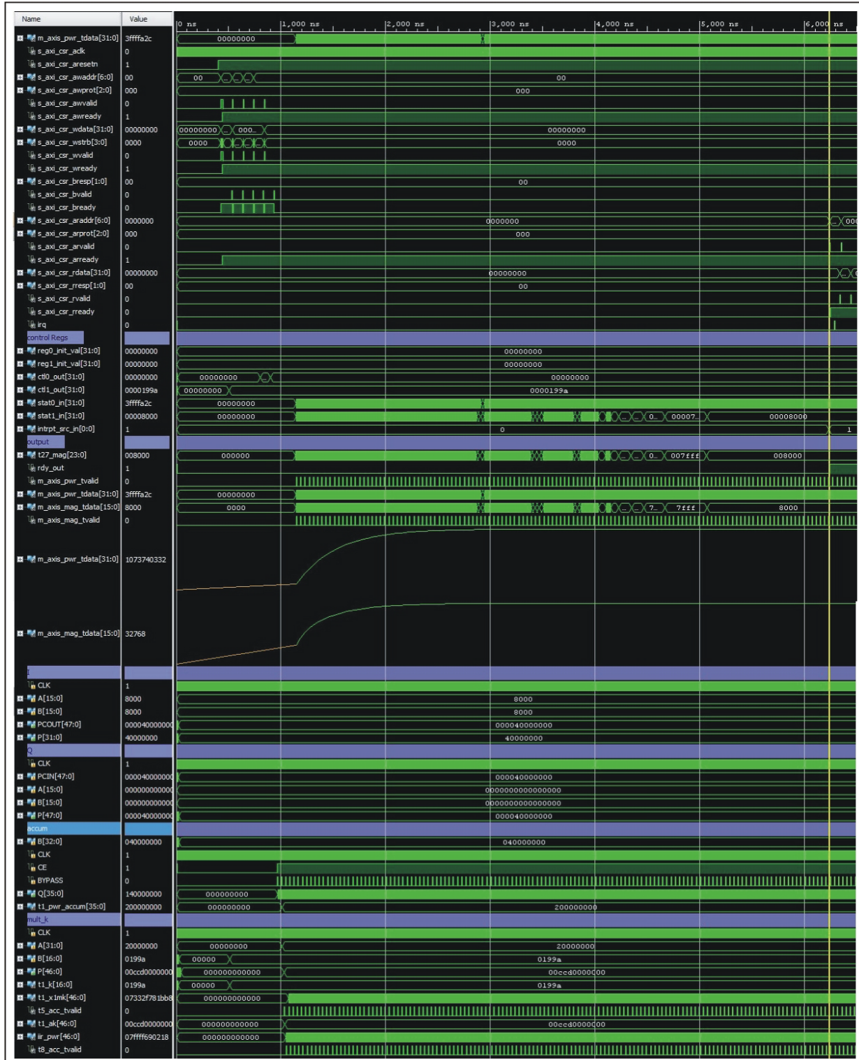
Figure 6-3: AXI4-Stream Power Meter Core Test Bench Simulation Output
