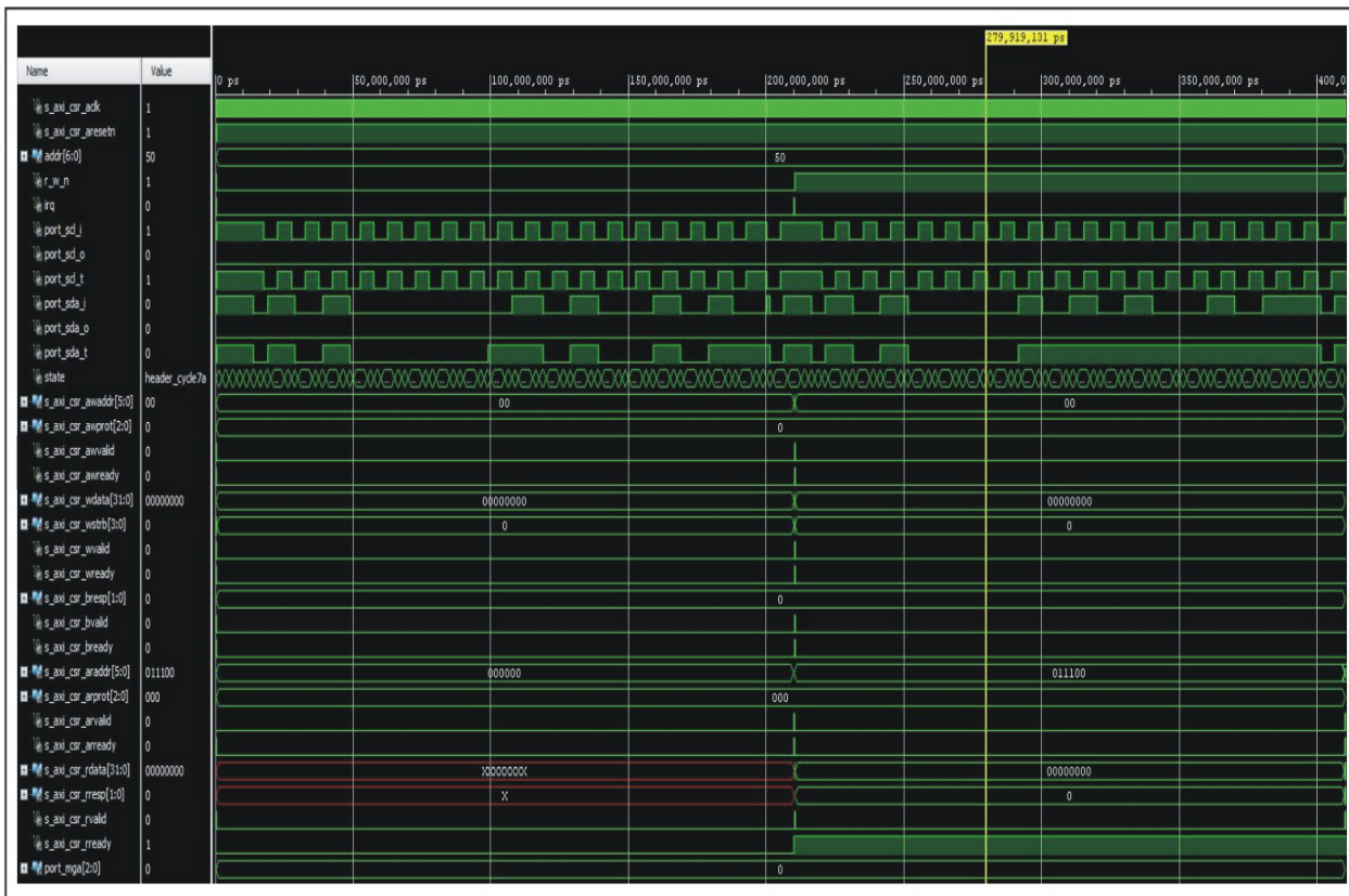
Figure 6-3: AXI I2C Bus Interface Core Test Bench Simulation Output
