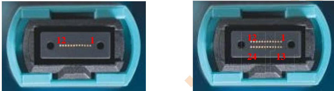
Figure 33: Fiber Numbering Convention for 12F and 24F Connectors
