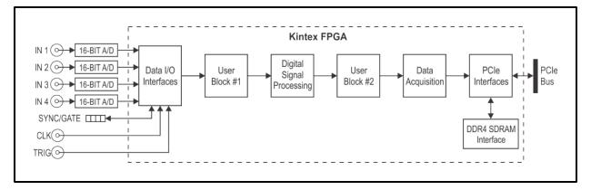
Refer to "FPGA IP Core Operation" on page 51 for a description of each of the top-level functional blocks of the FPGA IP code.
