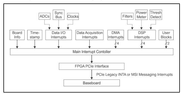
The block diagram below illustrates the interrupt signal routing on Model 71861.
