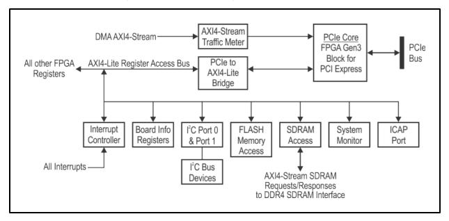
The memory map for these FPGA IP Core modules is provided in "PCI Express Interfaces" on page 71. For information about the corresponding support software, refer to "Board Support Software: Navigator Design Suite" on page 13.
