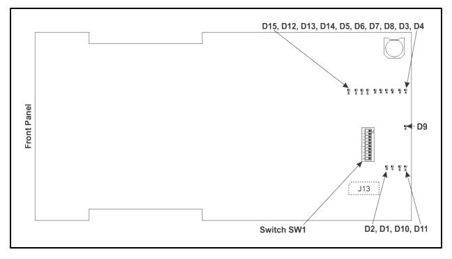
Switch **SW1** controls access to the FPGA configuration functions. The table below shows the settings for this switch.
