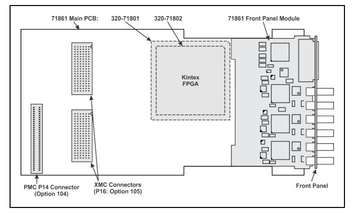
Note that a heat sink can be mounted on the Model 71861 PCB assembly as shipped.
