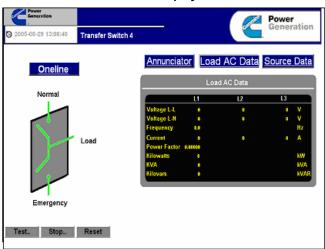
This screen graphically shows the status of the transfer switch by depiction of the connected source with the normal source and generator source switches shown as either open or closed. The display also provides tabular data covering the individual phase voltage, individual phase load current, power factor, frequency, kW, kVA, and kW hours. The screen also allows manual testing and fault reset of the transfer switch.
