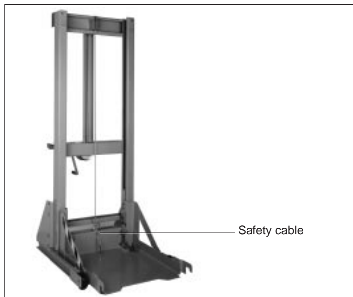
Figure 30: Circuit breaker lift truck
