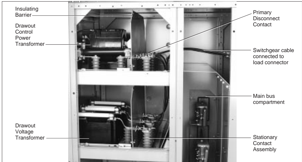
Figure 14: Drawout units in connected position
