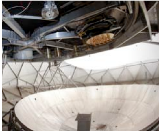
Figure 10. BYU's 19-element single-pol PAF mounted under the rotary floor of AO for the FOV Experiment.
