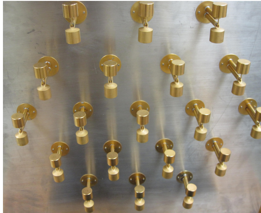
Single Polarization 19 BYU Dipole PAF
