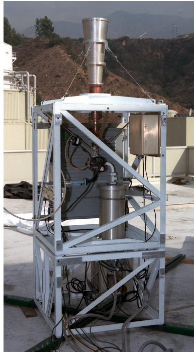
Fig. 7-24. X-band test package in the 22-dBi feed-horn configuration for testing.
