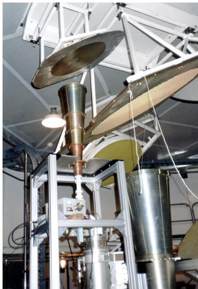
Fig. 7-47. DSS-13 S-/X-band feed-system geometry.
