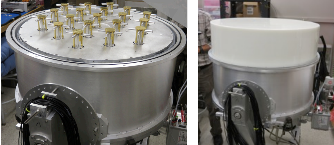
Figure 1.8: Left: New lower height metal vacuum shield installed on the AO19 cryo-PAF prototype. The dipoles have the new 0^\circ alignment (see Fig. 1.7). Right: AO19i dewar after installation of the HDPE “top hat” dome.
