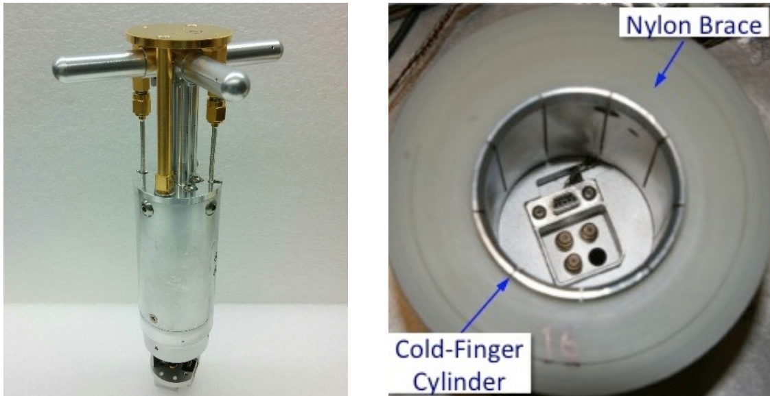
Figure 4.10: Left: Assembled dipole-LNA package with cylinder cover in place and blind-mate connector plug at the bottom. Right: View of cold-finger cylinder fixed on the 2 nd stage plate with nylon ring that braces firmly the dipole/package at cryogenic temperatures.
