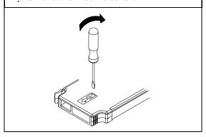
2 Connect wiring to the screw terminals.
