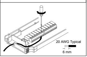
3 Route wiring through strain relief.
