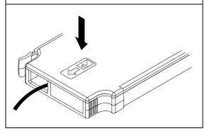
5 Install the module into mainframe.
