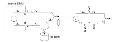
Two additional thermocouples have been created where the iron (Fe) lead connects to the internal DMM's copper (Cu) input terminals. Since these two junctions will generate opposing voltages, their effect will be to cancel each other. However, if the input terminals are not at the same temperature, an error will be created in the measurement.
