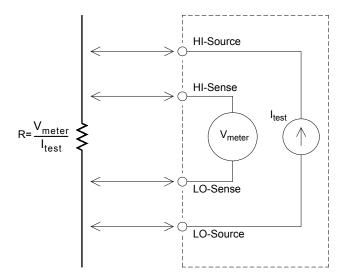
Offset Compensation Most connections in a system use materials that produce small DC voltages due to dissimilar metal-to-metal contact (thermocouple effect) or electrochemical batteries (for a description of the thermocouple effect, see page 262). These DC voltages also add errors to resistance measurements. The offset-compensated measurement is designed to allow resistance measurements in the presence of small DC voltages.
