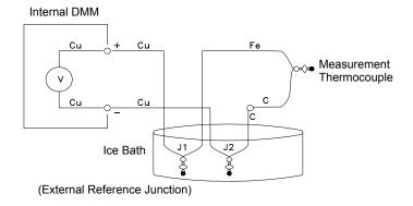
$This\ circuit\ is\ the\ best\ solution\ for\ accurate\ thermocouple\ connections.$
