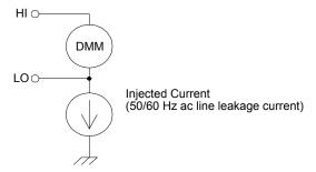
With  $Connection\ A$  (see below), the injected current flows from the earth connection provided by the circuit to the LO terminal of the internal DMM. This configuration adds no noise to the measurement. However, with  $Connection\ B$ , the injected current flows through the resistor R thus adding noise to the measurement. With Connection B, larger values of R will make the problem worse.
