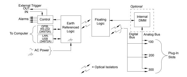
The earth-referenced and floating circuitry communicate with each other via an optically-isolated data link. The earth-referenced section communicates with the floating section to provide PC connectivity. The 34970A is shipped with both an GPIB (IEEE-488) interface and an RS-232 interface. Only one interface can be enabled at a time. The 34972A is shipped with Local Area Network (LAN) and Universal Serial Bus (USB) connectivity.
