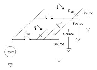
Capacitive noise coupling is a function of area and proximity. A simple method to reduce the noise coupling is to physically separate the switches and cables from each other. However, this may not be practical for all applications.
