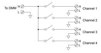
Note: Only one channel can be closed at a time; closing one channel will open the previously closed channel.
