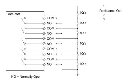
In the above diagram, the resistance is  $60\Omega$  when all of the actuator channels are open (not connected to COM). Note that when the actuator channels are open, as shown above, the normally-closed contacts (not shown above) are connected to COM. Values from  $10\Omega$  to  $50\Omega$  are selected by closing the appropriate channel(s) on the module.
