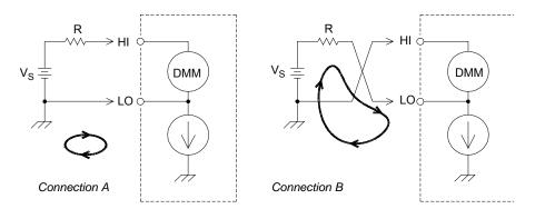
The measurement noise caused by injected current can be significantly reduced by setting the integration time of the internal DMM to 1 PLC or greater (see page 120 for a discussion of integration time).
