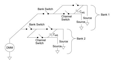
If you are not using all of the channels on the multiplexer, divide the input signals equally between Bank 1 and Bank 2. For example, if you are multiplexing eight channels using the 16-channel multiplexer, use four channels in the lower bank and four channels in the upper bank. For even better noise immunity, leave one unused, grounded channel between each input channel.
