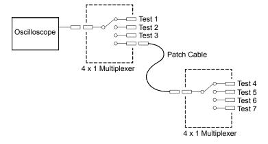
On the 34905A ( $50\Omega$ ) and 34906A ( $75\Omega$ ) RF multiplexers, you can close only one channel per bank at a time; closing one channel in a bank will open the previously closed channel. These modules respond *only* to the CLOSE command (OPEN does not apply). To open a channel, send the CLOSE command to another channel in the same bank.
