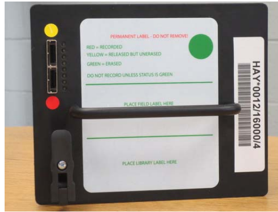
Figure 3: Disk-module labeling and mini-SAS cable connections; color codes must match.
