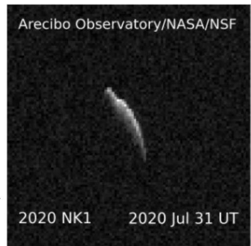
Figure 3: Radar delay-Doppler image of 2020 NK1 with vertical delay resolution of 0.05 \mu\text{s} (7.5 m) showing an elongated shape approximately 1km (0.6 mi) along the long axis.
