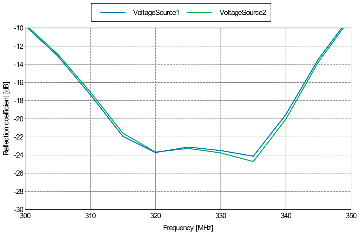
Figure 3: Reflection coefficient Magnitude - Crossed Dipole Feed Ref 4ft Dia .25 in Cyl Elements Opt2_optimum
